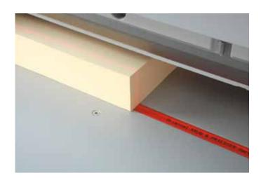
OPTICAL CUTTING LINE The optical cutting line with bright, durable LEDs shows where the cut will be performed and helps to align cutting marks precisely for accurate cuts.
