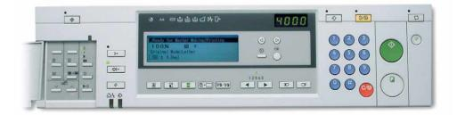
The large LCD control panel displays text and graphic icons for easy and confident user operation.
